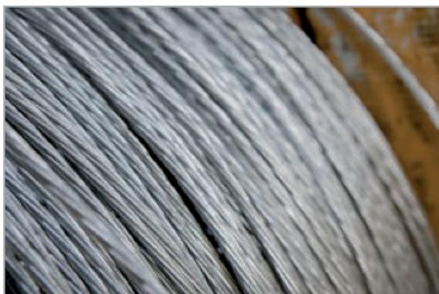
TORÓN 270 K SI/190 Kg/mm<sup>2</sup> - NORMA ASTM A-416
